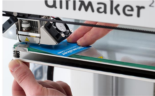
Prepare your plate for the perfect 1st layer by following your 3D printers bed calibration method (make sure to do it properly and maybe even 2 times)
