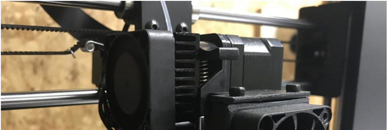
Example of a spring-loaded direct drive
