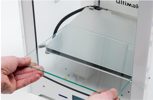
Make sure you have a clean glass plate (free of any oils / greases)
